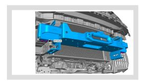
Install the winch armature assembly lower bolts.
